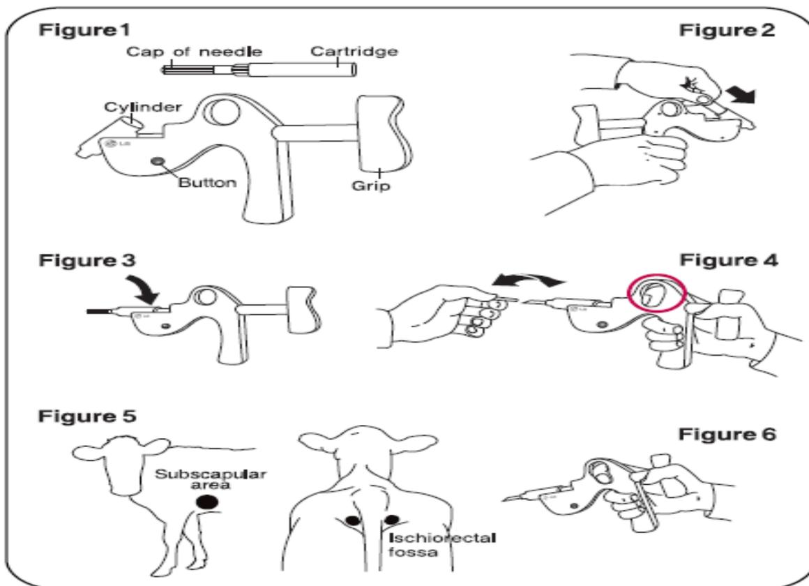
**Diagram:** Assembly of the cartridge and injector
